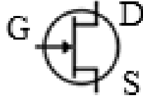
Fig. 7. Transistor: D – drain, S – source, G – gate.
